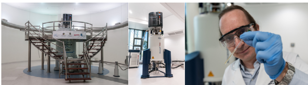
Figure 4: The flagship instruments of the UQ facility for NMR-based metabolomics are a 900 MHz ( left ) and a 700 MHz NMR spectrometer ( middle ). The facility is managed by Horst Joachim Schirra ( right ).
