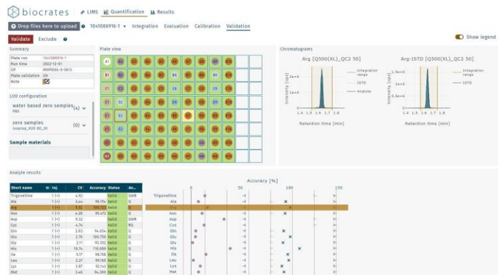
Figure 3: Plate validation – Calculation of accuracies and CVs for quality control and performance check
