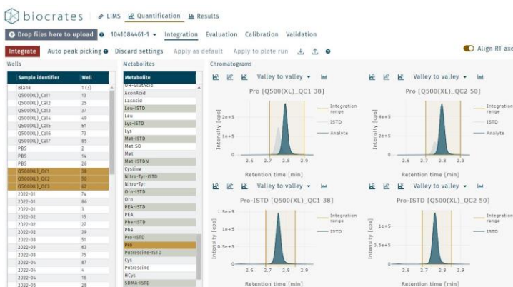
Figure 2: Automated peak picking and multiple view options allow fast peak integration and review
