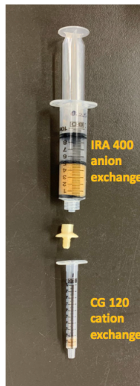
Ion-Exchange Chromatography Unit for Cleaning of Urine and Enrichment of the Metabolite Concentration
